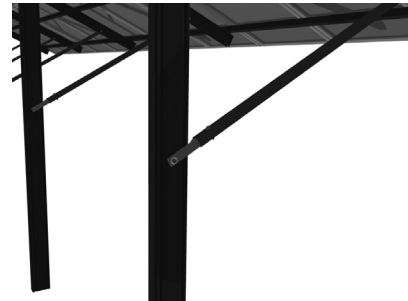
Linking of the diagonal to the C-post
